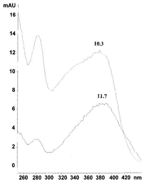
Figure 5. Diode array spectra of major products (named by retention time) derived from HPLC measurements after 60 min of reaction in model solutions containing chlorogenic acid (CG), (-)-epicatechin (EPI), lettuce polyphenol oxidase (PPO), and acetate buffer (pH 6.0, 30 °C) saturated with 80% O 2 , 0% CO 2 , and 20% N 2 . Absorbance is expressed as milliabsorbance units (mAu). For further details, see HPLC Measurements under Materials and Methods.
